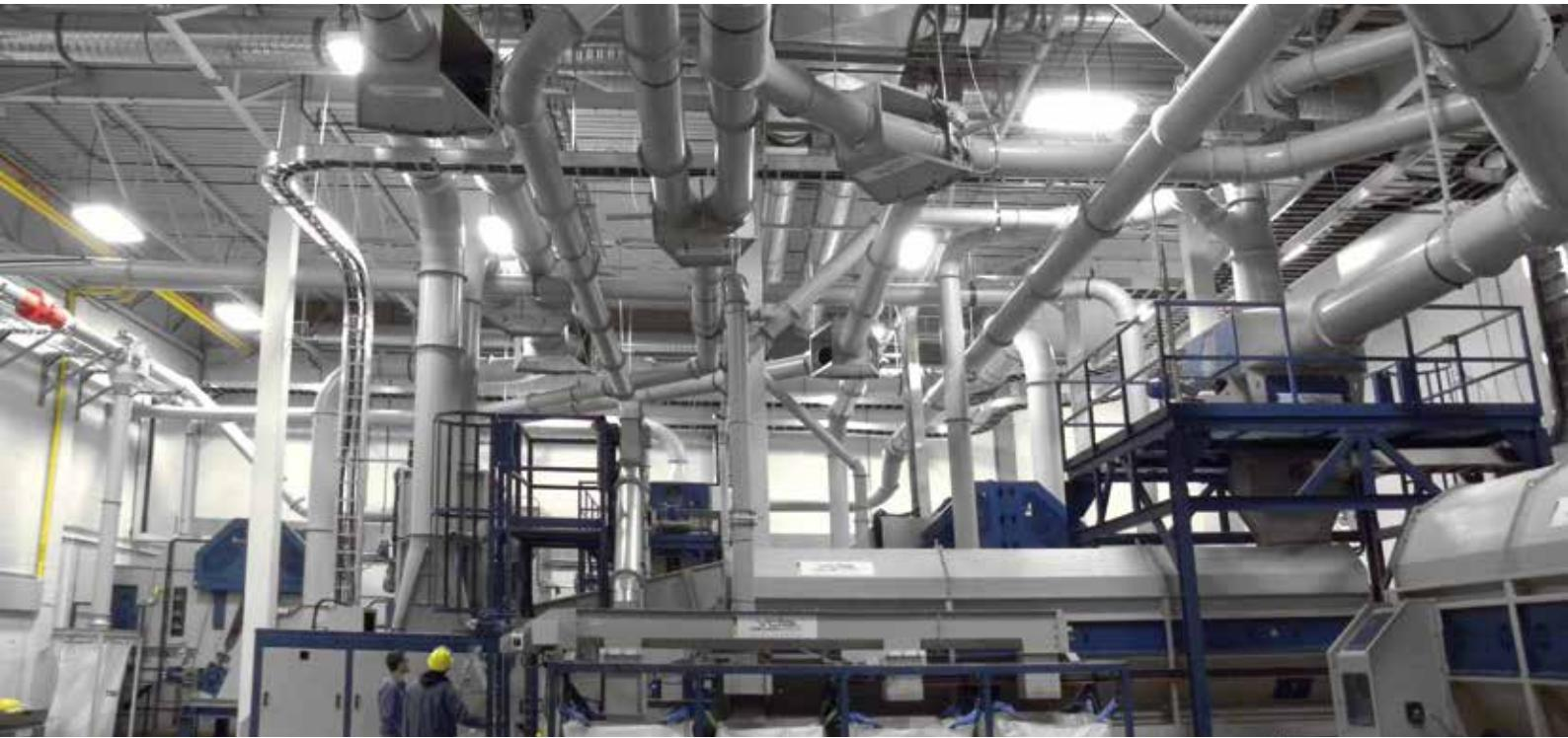
**EN** Processing of natural fibres – Turnkey projects for the harvesting and transformation of natural (bast) fibres such as flax, hemp, kenaf or similar. Feeding and opening of round or square bales. Separation of the fibres and the wooden core (shives). Extensive cleaning of the fibres and shives.
